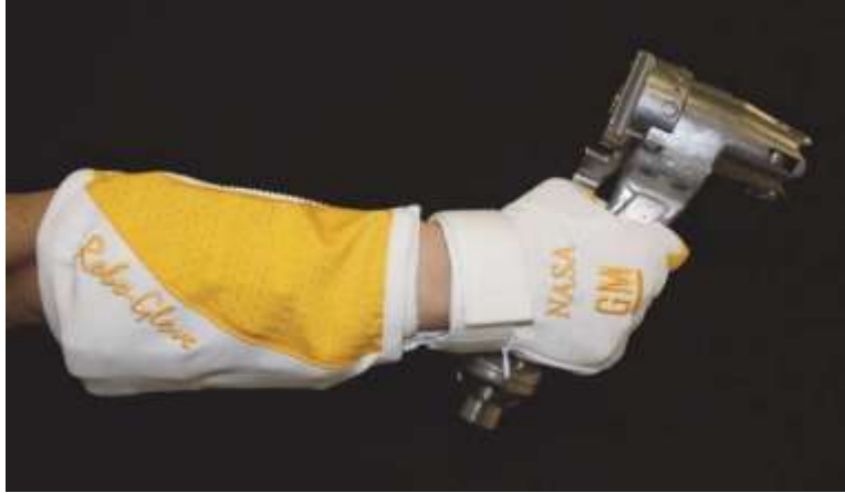
Fig. 1. The NASA/GM RoboGlove (shown here holding an example tool).
