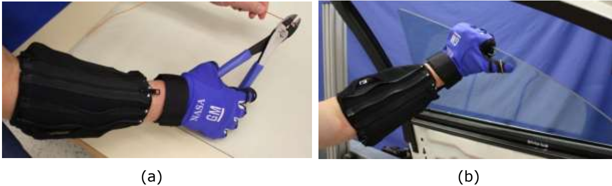
Fig. 3. Examples of (a) crimping and (b) door glass installation using RoboGlove (illustration only).
