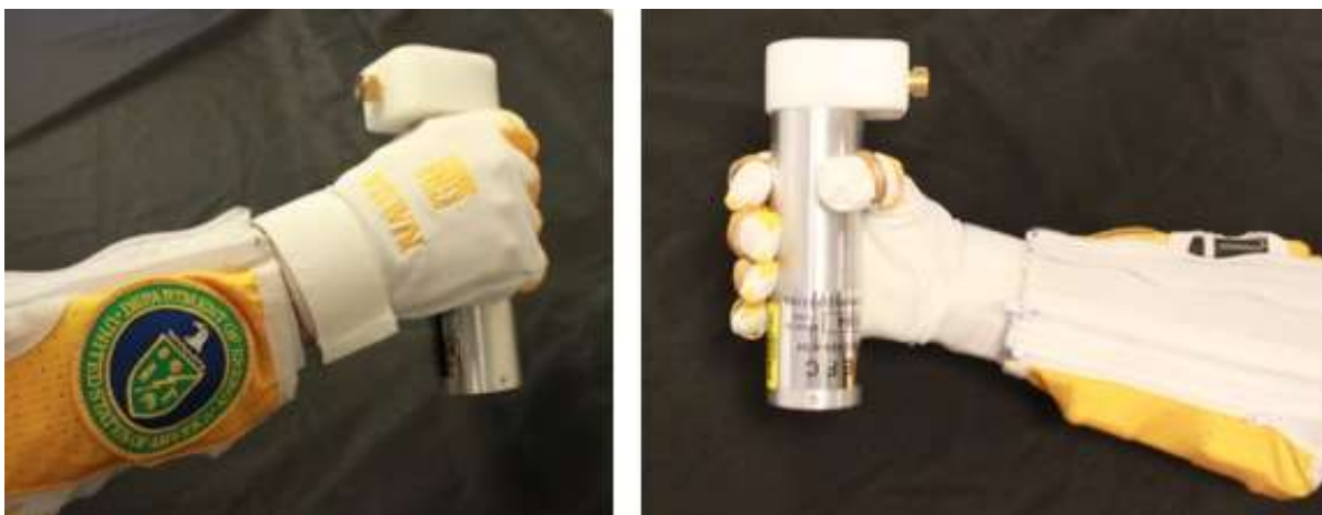
Fig. 6. Two images of RoboGlove-assisted manipulation of the HMS4 sodium-iodide radiation detector.
