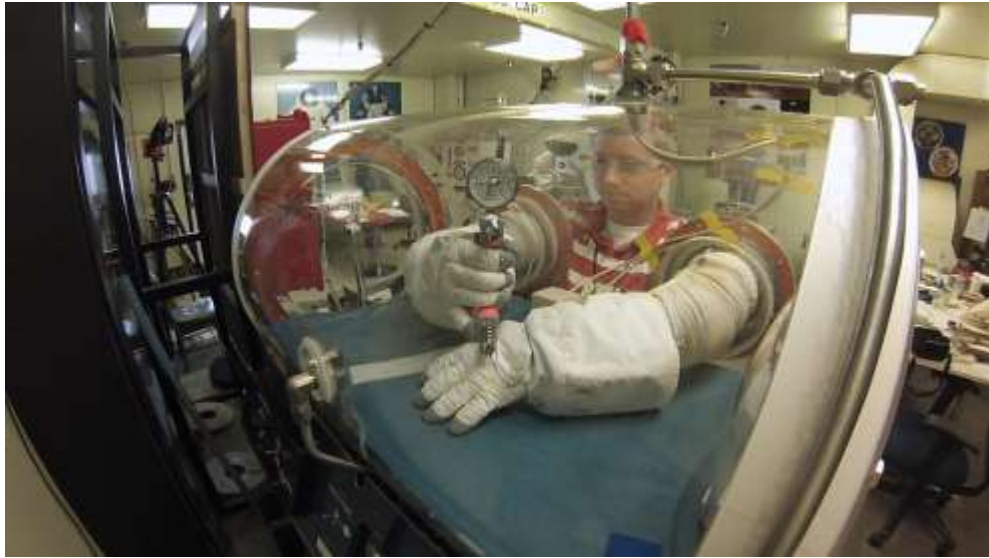
Fig. 4. Glovebox Testing of the Space Suit RoboGlove.
